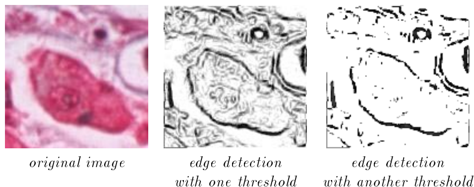
Figure 6.9: Automatic object segmentation of pathology images is an extremely difficult task. When different thresholds are provided, an edge detector either gives too many edges or too few edges for the object grouping. We avoid the precise object segmentation process by using our IRM “soft matching” metric.
