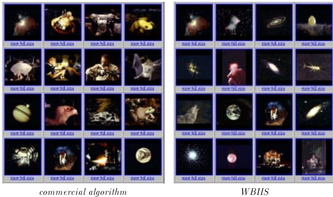
Figure 5.4: Comparisons with a commercial algorithm (IBM QBIC) on a galaxy-type image. Note that 12 out of 15 images retrieved by the commercial algorithm are unrelated to the galaxy query image. WBIIS retrieved only 6 unrelated images. The upper-left corner image in each block of images is the query. The image to the right of that image is the best matching image found. Matches decrease in measured closeness from left to right and from top to bottom. Results were obtained from a database of approximately 10,000 images.
