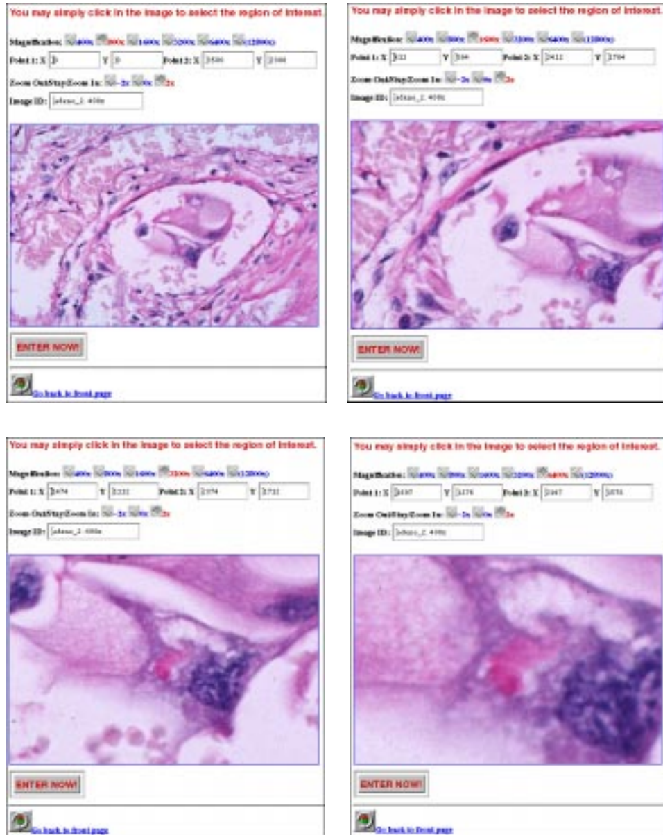
Figure 7.5: Multiresolution progressive browsing of pathology slides of extremely high resolution. HTML-based interface shown. The magnification of the pathology images are shown on the query interface.
