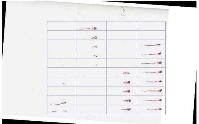
Fig. 3. Output from our algorithm: The lattice overlaid on the rotation-corrected input array image is detected by exploiting the topological 2D lattice structure and maximizing bilateral symmetry of the zebrafish larva in each lattice unit cell.
