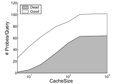
Figure 5: Number of dead probes increases as cache size increases, while good probes experience a maximum at moderate cache value
