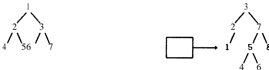
Figure I — Balanced trees in which a search for k takes O(\log k) time
