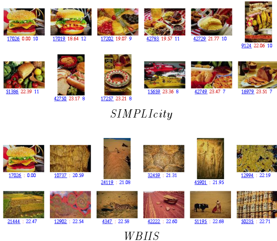
Figure 4: Comparison of SIMPLicity and WBIIS. The query image (upper-left corner) is a photo of food. Best 11 matches are shown.
