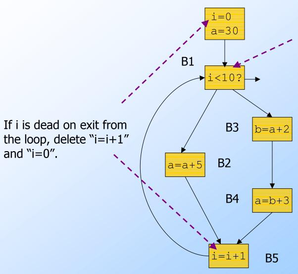
Here, the value of a is m(a)+5i, where m(a) is the value of a before entering the loop, and i is the number of iterations of the loop so far.
