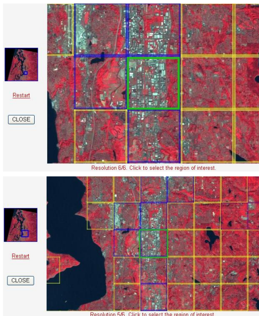
Figure 3: Interface for zooming, showing urban (blue), residential (yellow) and the retrieved (green) patch. Top : Original 30m resolution. Bottom : Zoomed out at 60m.
