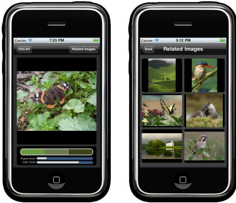
Fig. 2 User interface of OSCAR mobile application. Left: photo submitted to the server, best color triplets and its confidence score, aesthetics score of the photo (scores are indicated by bar). Right: similarly composed exemplars retrieved from the database.
