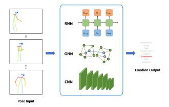
Fig. 15. Skeleton-based BEEU takes the 2-D/3-D pose sequence of the target human instance as input.
