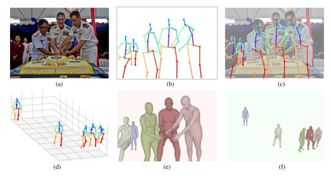
Fig. 6. Example of state-of-the-art deep learning-based human pose and mesh detection with individuals in the scene separated properly [102]. The input to the methods is a standard 2-D RGB photograph. The 3-D mesh method provides an estimation of the relative depths of the people in the scene. (a) Original photograph. (b) 2-D pose. (c) 2-D pose, superimposed. (d) 3-D pose. (e) 3-D mesh. (f) 3-D mesh, alternative view.
