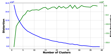
Fig. 10: The result of the elbow method on the dataset. We could spot the elbow around 13-17 clusters. We are also showing the first derivative of the distortion, to show where it is going to flatten out.
